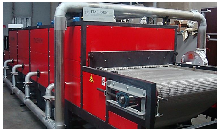
FORNO A TAPPETO IF/RE/5/1000 - Placchette in silicio TAPE KILN IF/RE/5/1000 - Silicon plates
