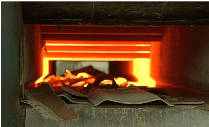
FORNO A RULLI OK 42/2400 - Inertizzazione amianto ROLLER KILN OK 42/2400 - Inertization of asbestos
